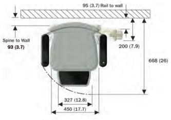
Measurements are in millimetres. Measurements in brackets are inches. All dimensions measured from the wall are nominal. The addition of a wide stringer or similar obstruction may affect the dimensions taken from this point. The colour representation of the chair shown here is for illustrative purposes only. Weight limit note: Upto 135kg - approx 21 stone
