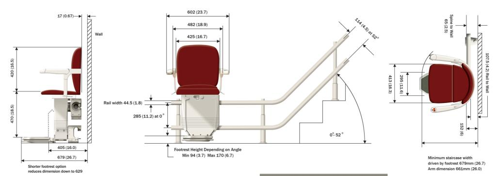
Measurements are in millimetres. Measurements in brackets are inches. All dimensions measured from the wall are nominal. The addition of a wide stringer or similar obstruction may affect the dimensions taken from this point. The colour representation of the chair shown here is for illustrative purposes only. Weight limit note: Upto 135kg - approx 21 stone / 297 lbs. Powered hinge is limited to 120kg - approx 19 stone / 265 lbs.
