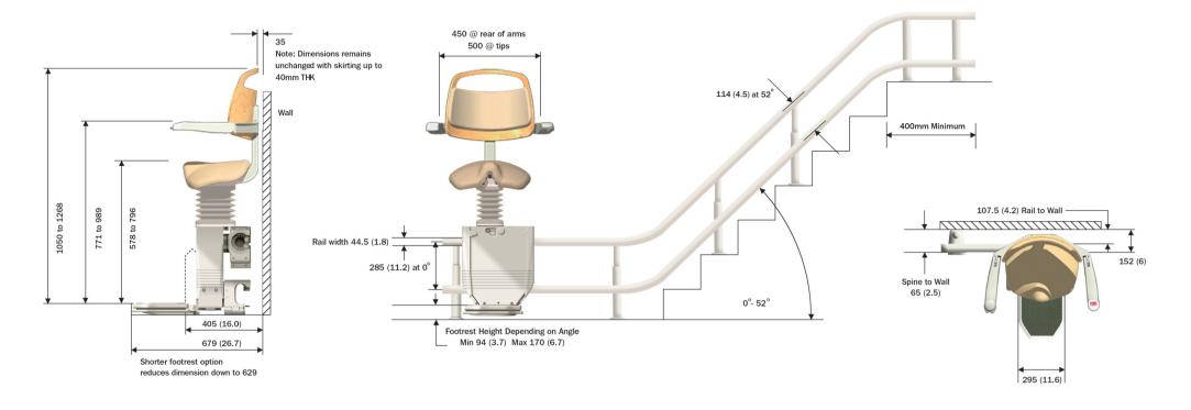
Measurements are in millimetres. Measurements in brackets are inches. All product dimensions are accurate, however, you should add approximately 25mm on dimensions that require clearance to the opposite wall, such as minimum staircase width driven by footrest in the down position.
